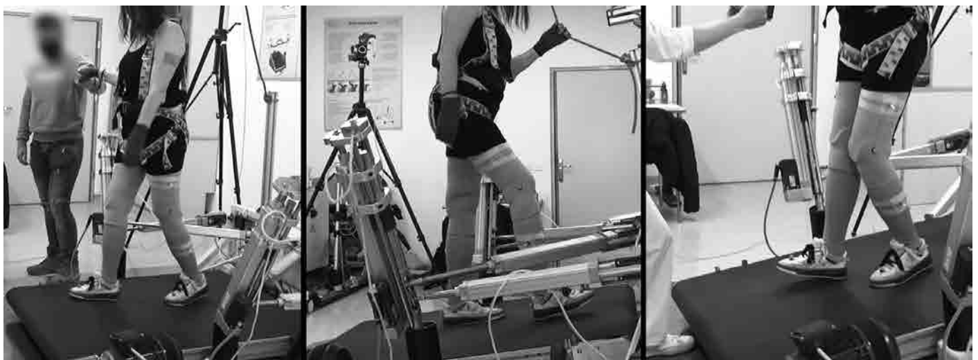
Figure 1: Bilateral transtibial amputee walking on a flat, uphill-sloped and downhill-sloped instrumented treadmill.
