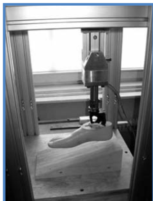
Figure 1: Testing device for oscillation response of the heel
