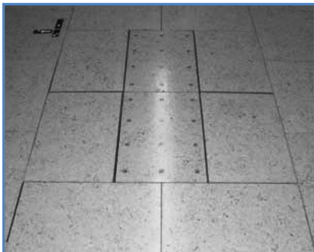
Figure 3: Flat surface with two force plates
