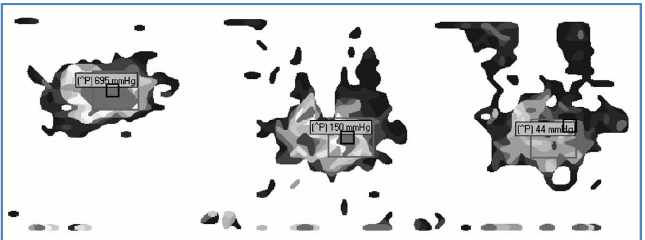
Figure 2: Example of Tek Scan seat pressure mapping for standard chair, custom seat cushion and modified custom seat cushion.
