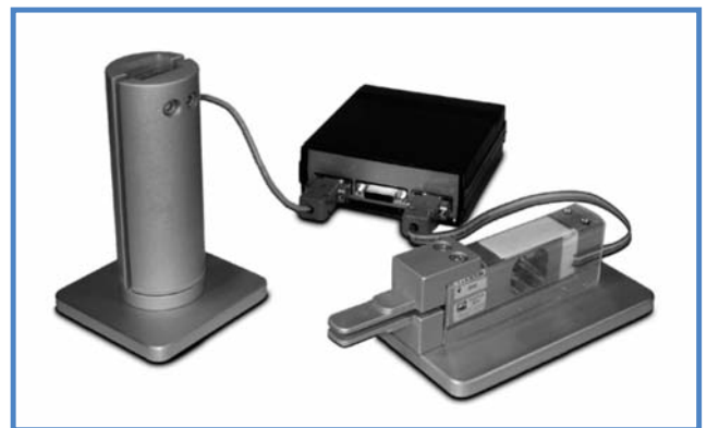
Figure 1: A compact assessment system with two force measuring units in the shape of a cup and thin plate can be connected to a personal computer to accurately measure the dynamic grip force in cylindrical and lateral grip.
