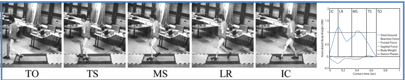
Figure 9: Detected stance phases of pathologic subject's left leg (LR: 0.14 sec, MS: 0.26 sec, TS: 0.38 sec, TO: 0.68 sec)
